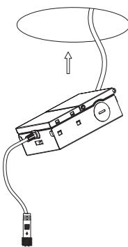
3. PLACE ALL WIRING AND CONNECTIONS BACK INTO THE J-BOX AND CLOSE THE COVER AND INSERT THE J-BOX THROUGH THE MOUNTING HOLE.
