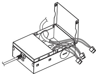
2. OPEN THE J-BOX COVER AND REMOVE THE APPROPRIATE KNOCKOUT(S). INSERT THE ELECTRICAL SUPPLY CABLE THROUGH THE KNOCKOUT AND SECURE WITH A CABLE CONNECTOR (SOLD SEPARATELY). USING PUSH-IN WIRE CONNECTORS AND CONNECT THE WIRE.
