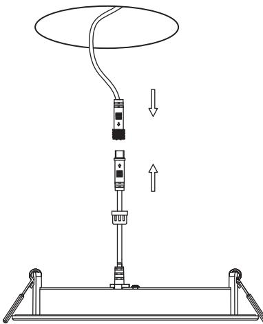
4. CONNECT THE FIXTURE BY INSERTING AND TWISTING THE MALE/FEMALE CONNECTORS
