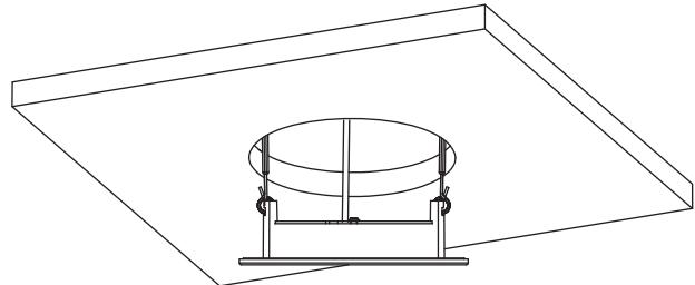
5. PUSH SPRING LOADED CLIPS ON THE FIXTURE UPWARDS AND INSERT THE FIXTURE INTO THE MOUNTING HOLE. RELEASE THE CLIPS AND THE FIXTURE WILL BE PULLED FLUXH TO THE CEILING.
